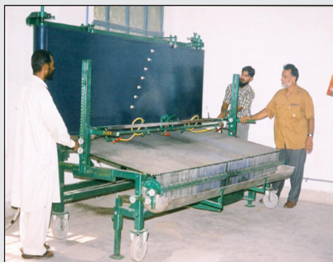
For under spraying, inserting water sensitive papers in WSP holders on Vertically moving platform of Boom Sprayer Test Bench
